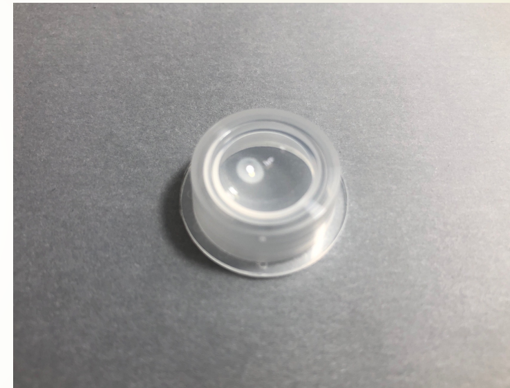
Spin cast molding - plastic optical mold
